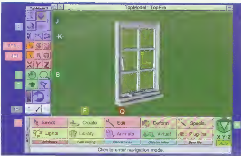
Figure 1: Breakdown of TopModel2's user interface showing the location of functional groups and key features mentioned in the text. These include tools for navigation (green), object manipulation (red), object creation (yellow), general information (cyan), animation (pink) and altering the environment (blue)
